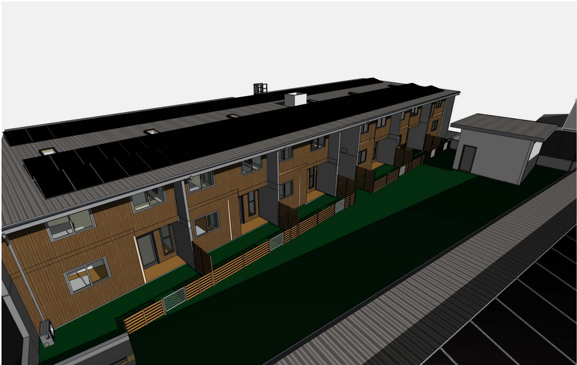
Shadow Diagram - Southern Units, North Elevation June 21, 11.00 am
